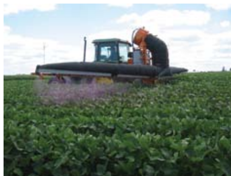
Drop cards in the canopy measure droplet size (top). An air-assisted sprayer places pesticide in the lower parts of the plant canopy (bottom).
