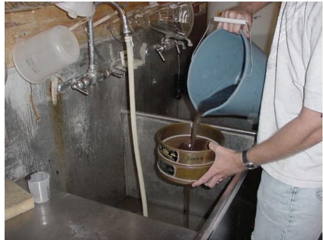
Separating nematode worms or cysts from soil sediments by sieving soil-water suspension. (Greg Tylka)
